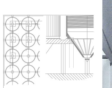
Floor with building columns of reinforced concrete; 4 supports for each tank; particularly suitable for very large tanks
