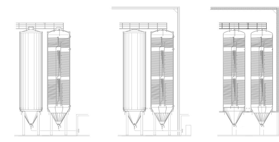
Insulated tank on pipe columns, connected to operator aisle in the building
